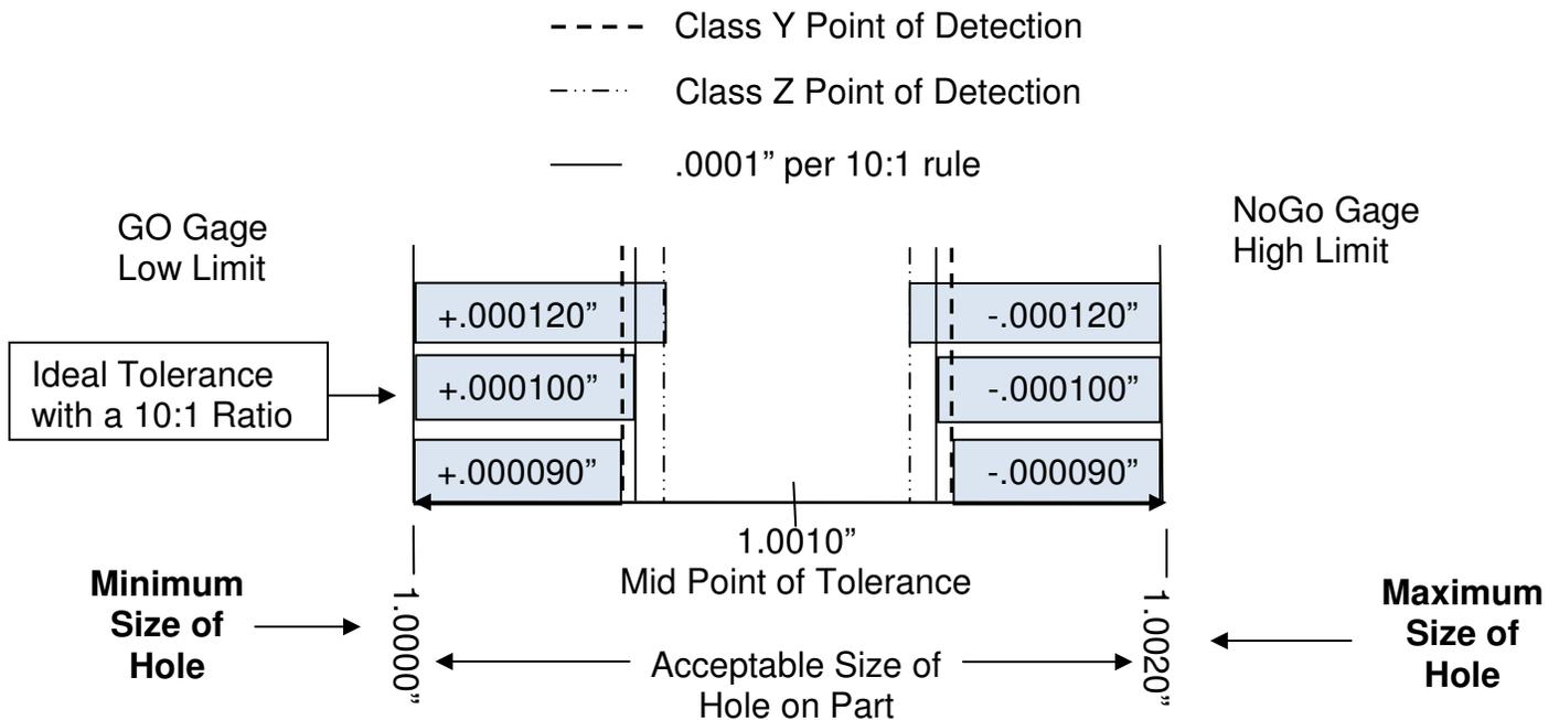
At this point it is a good time to discuss risk vs. cost of scrap. As depicted in the above figure it becomes obvious that the less accurate plug gauge will detect an out of tolerance condition sooner than the more accurate gauge. And the less accurate gauge costs less.
